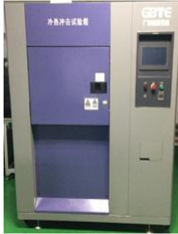
Thermal Cycling Testing
