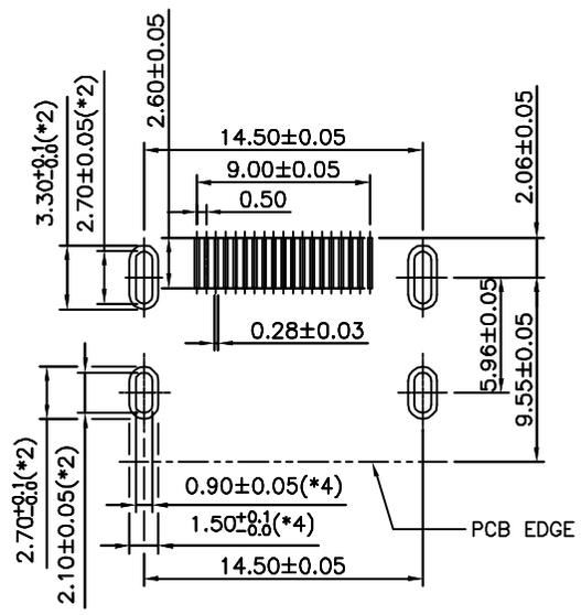
Recommended P.C.B Layout (Thickness=1.6±0.15mm)
